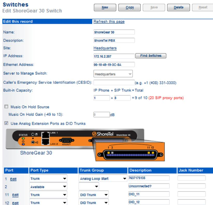
3. Select the number of SIP trunks from the ports available. Each port designated as a SIP trunk port type enables the support for five individual SIP trunks.
