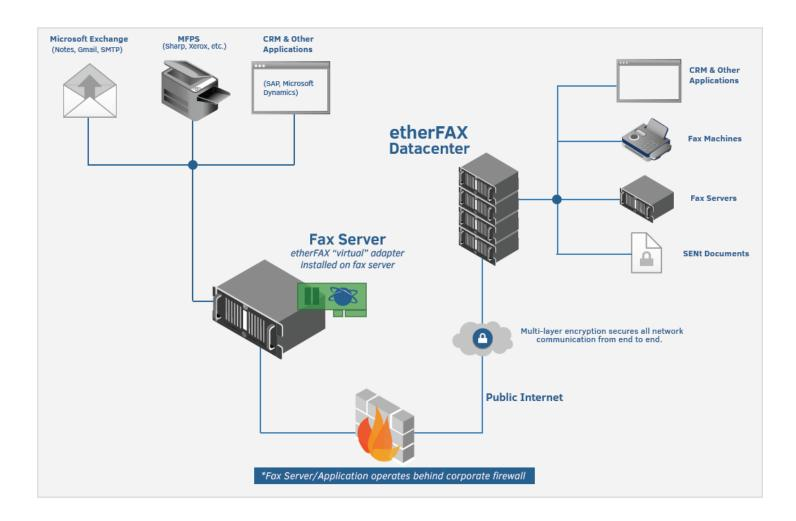
Once you submit a job to the FF240-IP, the documents are rendered and readied for transmission. Each fax is authenticated and securely delivered over HTTPS to its destination using etherFAX's carrier grade telephony network. The fax transmission is updated and monitored in real-time with final call progress notification sent to the FF240-IP and viewable on the fax status page.
